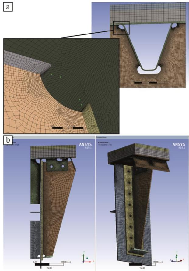
Figure 3. Submodelling. (a) Longitudinal stiffener; (b) Cantilever crossbeam.
