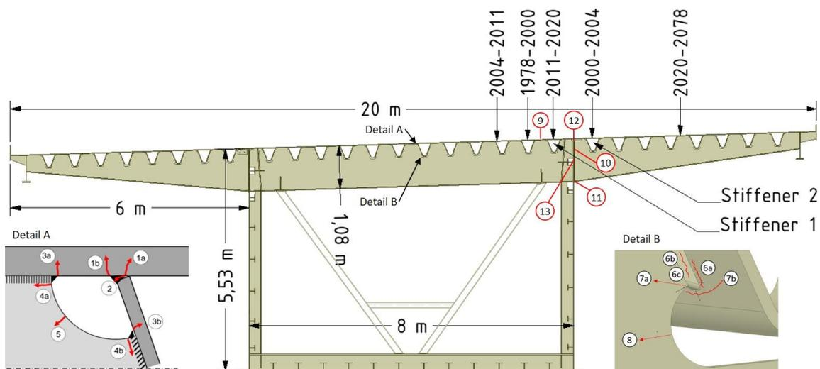
Figure 2. Global dimensions of the closed box girder including the fatigue details and historical truck positions (arrow represents the center of the right wheel of the trucks)
