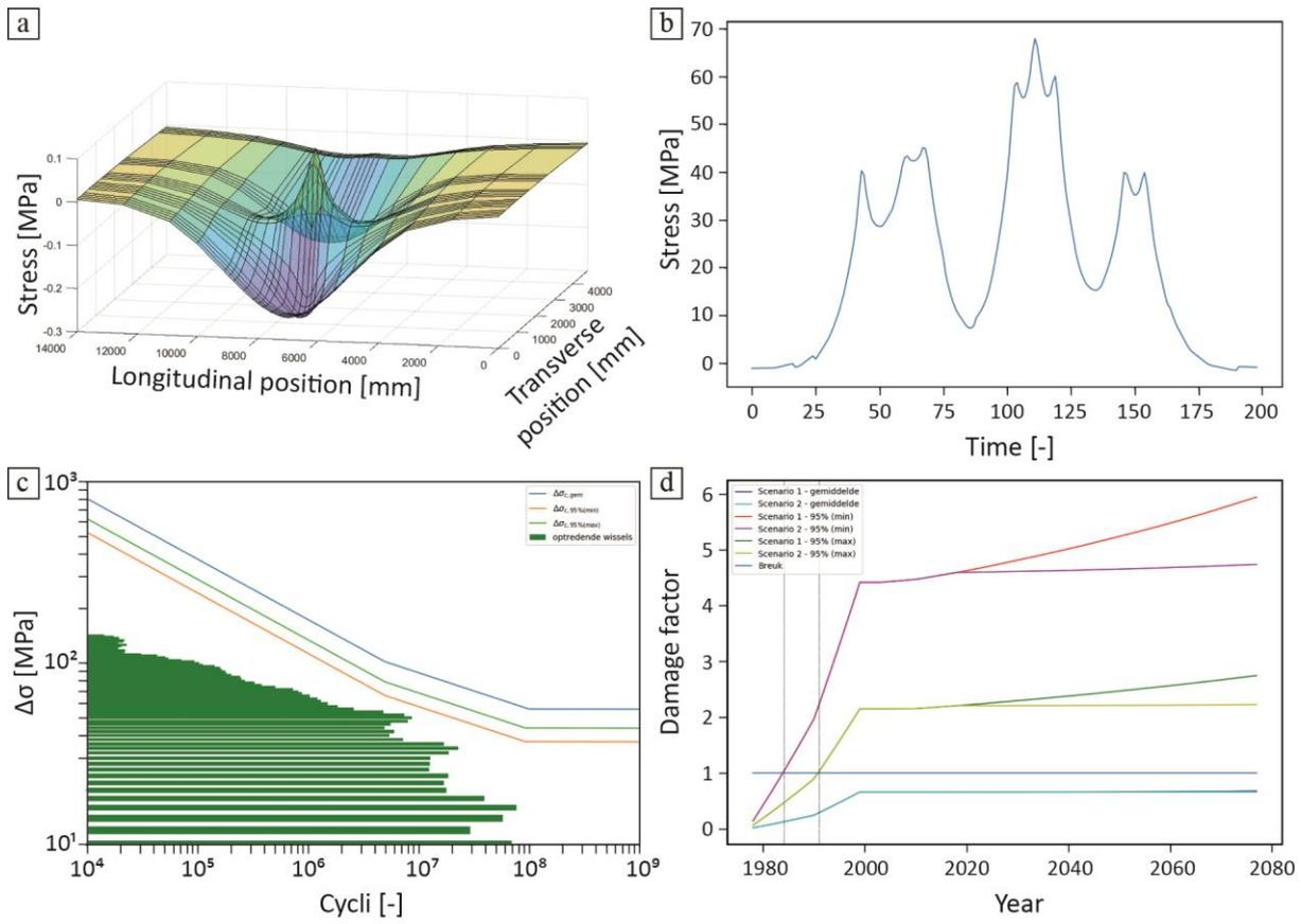
Figure 4. Post-processing flow. (a) Influence surface; (b) Stress variation due to a passing truck; (c) Total histogram of the stress cycle counting; (d) Fatigue damage curves in function of time.
